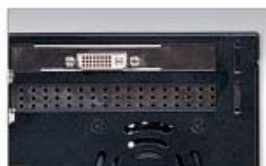
PCI Expansion One PCI expansion slot for adding more functions to the system
